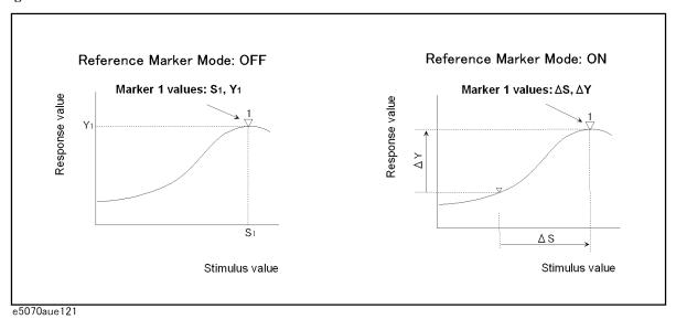
**Step 1.** Following Step 1 to Step 5 in "Reading Values on the Trace" on page 173, place the reference marker on the point to be used as the reference.
