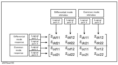
Figure 7-12 Mixed mode S-parameter when measuring a single-ended - single-ended - balanced device
