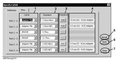
**Step 4.** For each test port, select a calibration kit you use (1 in Figure 4-33). In addition to the 10 calibration kits you can select for normal calibration, you can select Adapter File. When you want to use the adapter as the standard, select Adapter File.
