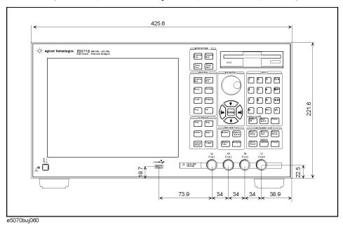
Figure 15-2 Dimensions (front view, E5071B with Option 313, in millimeters, nominal)
