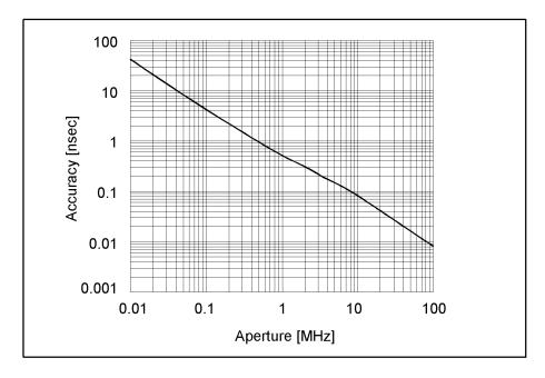
In general, the following formula can be used to determine the accuracy, in seconds, of specific group delay measurement:  $\pm \ \text{Phase Accuracy (deg)} \ / \ [360 \times \text{Aperture (Hz)}]$
