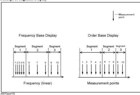
Figure 11-10 Comparing Methods of Displaying Segments
