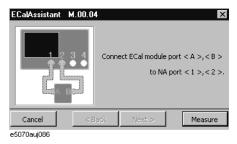
**Step 11.** Following the connection diagram shown in the dialog box (Figure 4-23), connect port A and B of the ECal module to test ports on the E5070B/E5071B.
