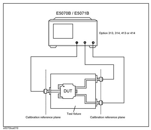
Figure 7-23 shows the measurement circuit simulated by the fixture simulator based on actual measurement with the test fixture shown in Figure 7-22.
