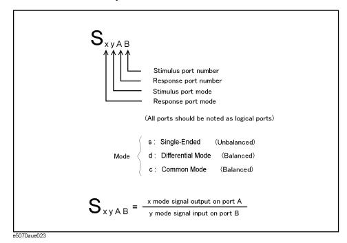
Figure 7-10 to Figure 7-12 show the mixed mode S-parameter when measuring each balanced device.
