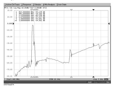
The measurement conditions are determined for each frequency range. Here, the segment sweep is performed following the sweep conditions shown in Table 14-2.
