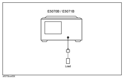
**b.** Press **Load (Optional)** to start the measurement on the LOAD standard.
