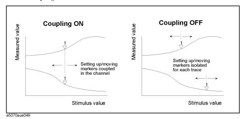
Marker Couple is on. (Coupling ON)
