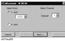
**Step 5.** Following the instructions in the dialog box, select the type of ECal, test ports, and a channel.
