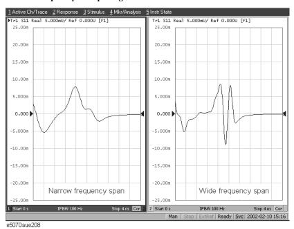
The sweep range affects the width of the impulse signal and the rise time of the step signal. The width of the impulse signal and the rise time of the step signal are inversely proportional to the sweep range. Therefore, the wider the sweep range is, the shorter these times are.
