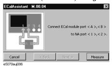
**Step 7.** Connect the ECal module to the test ports according to the instruction in the dialog box and then press **Measure**.
