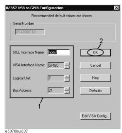
If you need to check/change the setting of the USB/GPIB interface after connecting the USB/GPIB interface, follow these steps:
