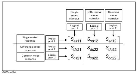
Figure 7-11 Mixed mode S-parameter when measuring a balanced - balanced device
