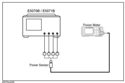
**Step 8.** Press **Take Cal Sweep** to start the measurement of calibration data.
