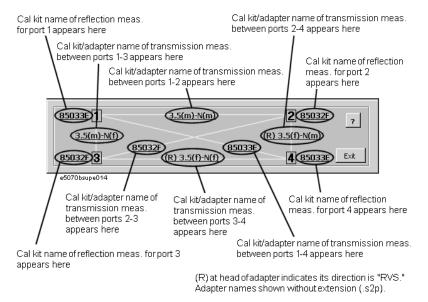
Calibration procedure in the adapter calibration mode is the same as that in the normal calibration except that the standard connected for each calibration data measurement differs. Therefore, when performing the calibration, you use the softkeys (the menu displayed by Cal - Calibrate) you use in the normal calibration.
