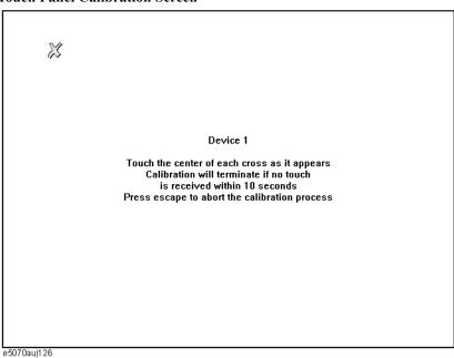
**Step 5.** Touch the x mark on the upper left with your finger. The mark x appears also on the lower left, upper right, and lower right. Touch the x marks in that order with your finger.
