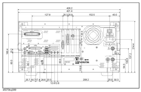
Figure 15-5 Dimensions (side view, in millimeters, nominal)
