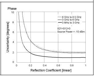
Table 15-5 Corrected System Performance With 3.5 mm Device Connector Type, 85093C Electronic Calibration Module
