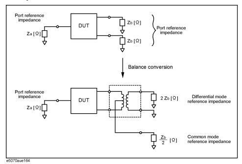
As described above, the impedance of the balanced port is automatically specified as the result of specifying the impedance of the two unbalanced ports prior to balance-unbalance conversion. However, the port impedance can be changed to an arbitrary value using the differential port impedance conversion function and the common port impedance conversion function.
