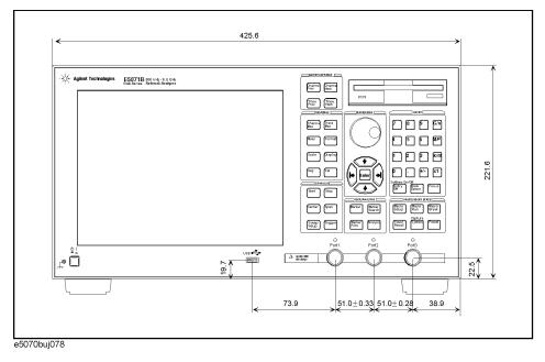
Figure 15-3 Dimensions (front view, E5071B with Option 213, in millimeters, nominal)
